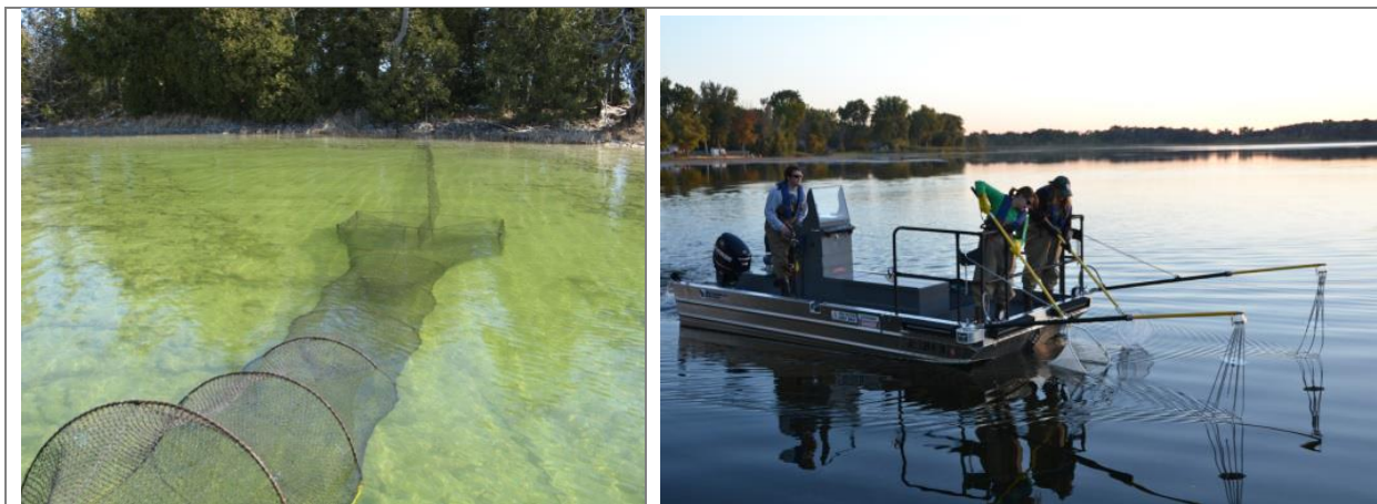
Photograph 3.5-1. Fyke net positioned in the littoral zone of a Wisconsin Lake (left) and an electroshocking boat (right).
